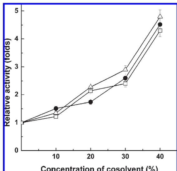
**Figure 1.** Relative activity of endoglucanase at its optimum temperature as a function of cosolvent concentration in 0.02 M sodium acetate buffer, pH 5.0. Sucrose (△), sorbitol (●), and glycerol (□).
