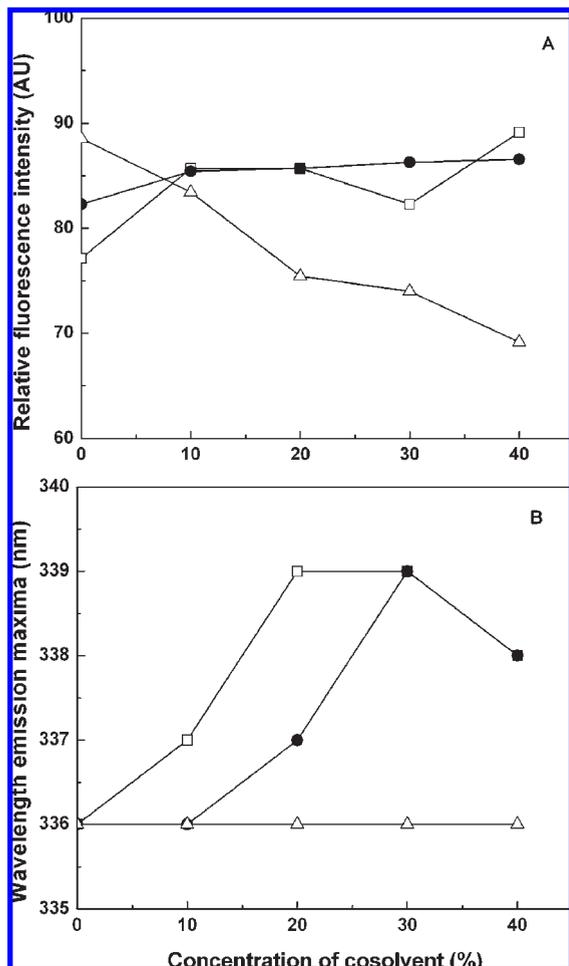
**Figure 4.** (A) Changes in the fluorescence intensity of endoglucanase as a function of cosolvent concentrations. (B) Changes in the fluorescence emission maxima of endoglucanase as a function of cosolvent concentrations. Glycerol ( $\square$ ), sorbitol ( $\bullet$ ), and sucrose ( $\triangle$ ).
