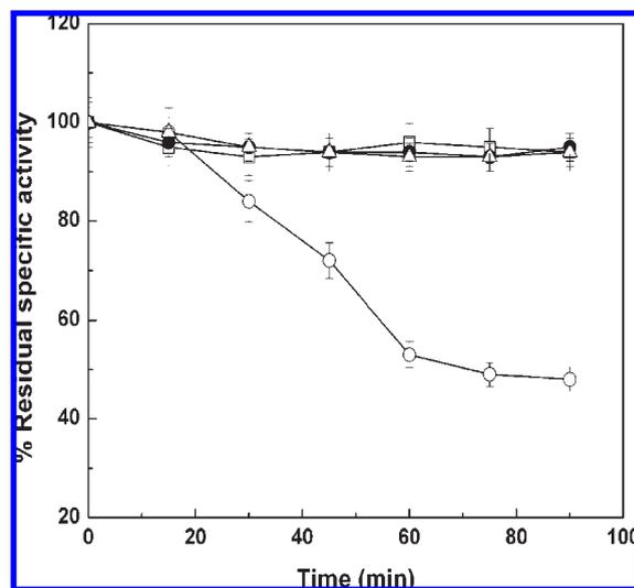
**Figure 2.** Effect of cosolvents on thermal inactivation of endoglucanase. The enzyme activity of samples heated at 90 °C with (40%) and without cosolvents was measured at pH 5.0 at 37 °C. Control (○), glycerol (□), sorbitol (●), and sucrose (△).
